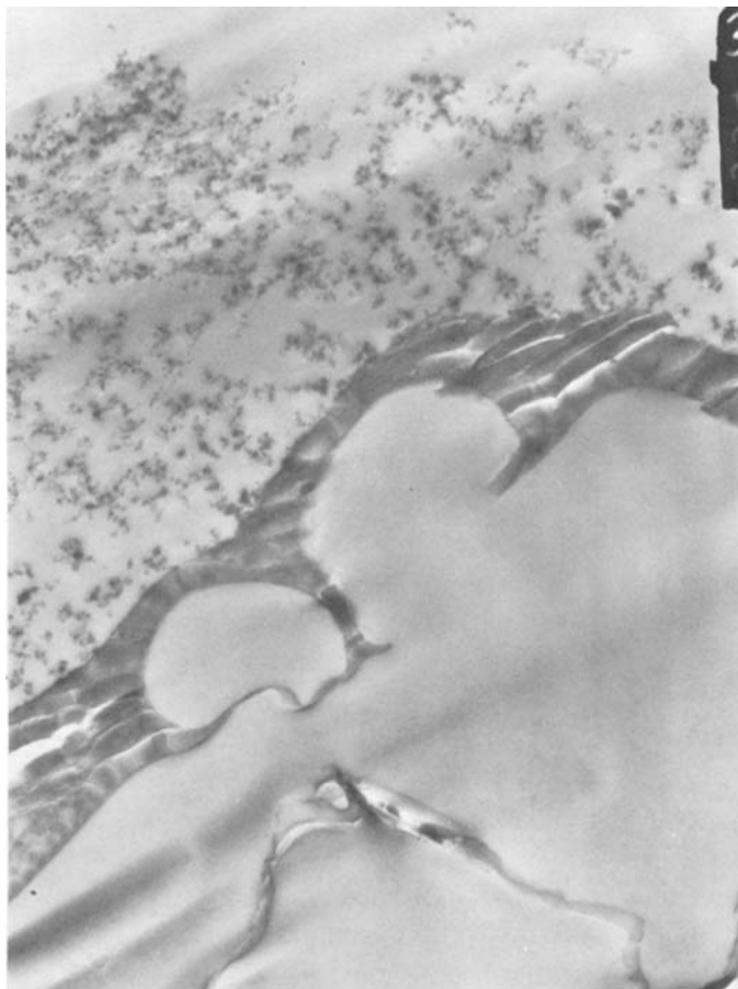
Fig. 15. Transmission electron micrograph of ultrasection of epoxy-impregnated LOI char from BPAC/DMS resin of 12% DMS showing friable electron-dense layers. 7500 \times .
