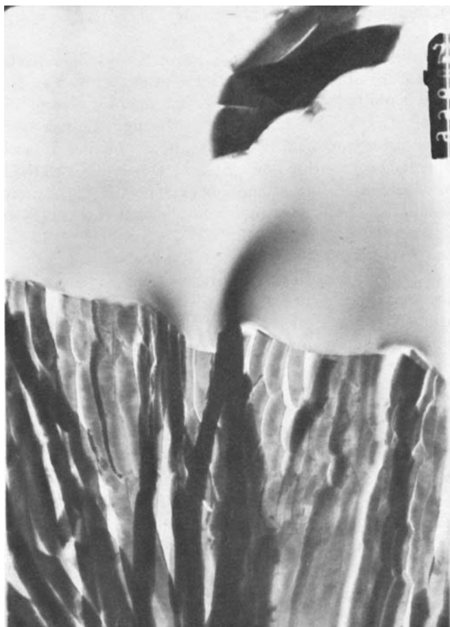
Fig. 16. Ultrasection of pyrolysis char from BPAC/DMS resin of 18% DMS showing char wall of same character as friable layers in Figure 15. 7500 \times .
