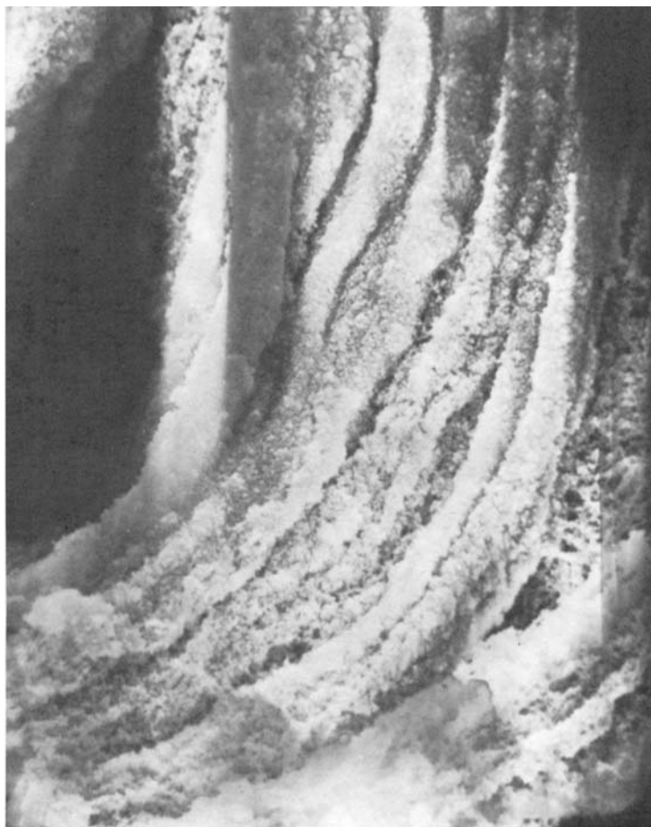
Fig. 7. Lamellar deposits of silica particles in surface of char of BPAC/DMS resin of 18% DMS burned out at OI = 41 (SEM). 1100 \times .
